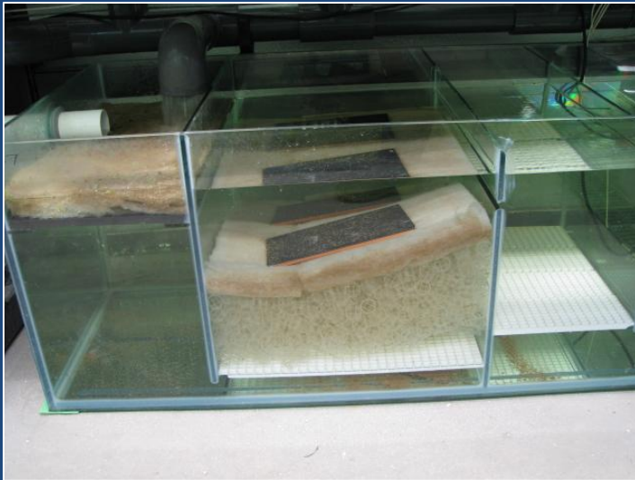
Mixture of biological and mechanical filtration
